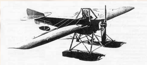
1/5 scale model of Nieuport monoplane on floats tested in the Auteuil wind tunnel on January 14, 1913, [4]
