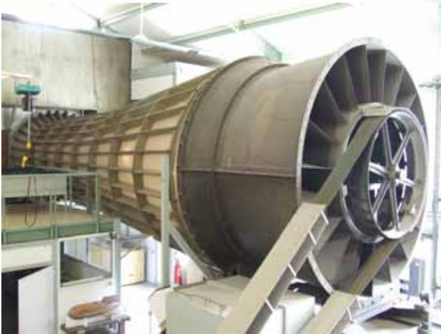
Blower at the discharge end of the tunnel, The Eiffel Laboratory; Author's personal collection
